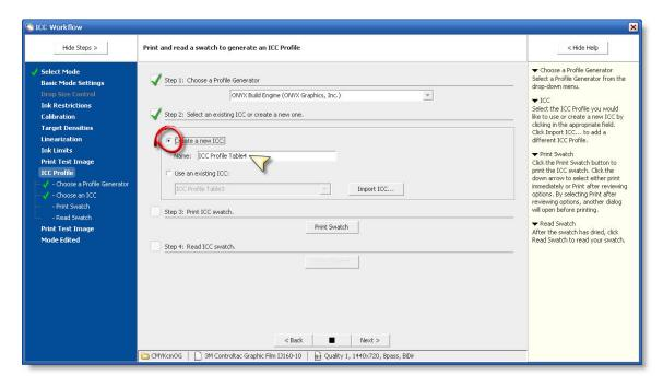
If you want to create a new Profile table, select the radio button 'Create a New ICC" and give the table a new name for example "ICC Profile Table 4"
