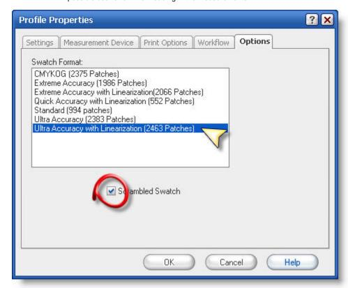
Note: The list of swatch formats matches the type of printer you are profiling. If you are profiling a CMYKOG Printer you must choose CMYKOG Patches and if you're profiling CMYKRGB Printer you must choose the CMYKRGB Patches.
