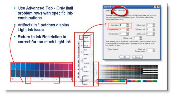
The numbers located on the left-hand side of the printed swatches correspond the the fields within the software. When evaluating the Ink Limit swatch, review each row or group of rows and keep the following in mind:
