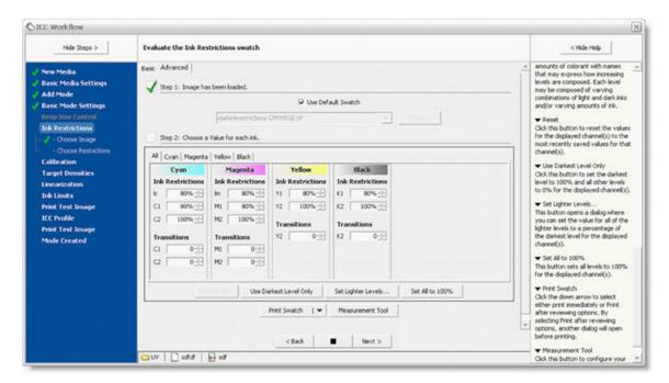
The Advanced Ink Restrictions option allows the user to add some refinement to the settings for Dark Ink restrictions, as well as a greater degree of control for setting Light Ink restrictions, or in the case of printers with multi-level dot size and/or multiple strike capabilities.
