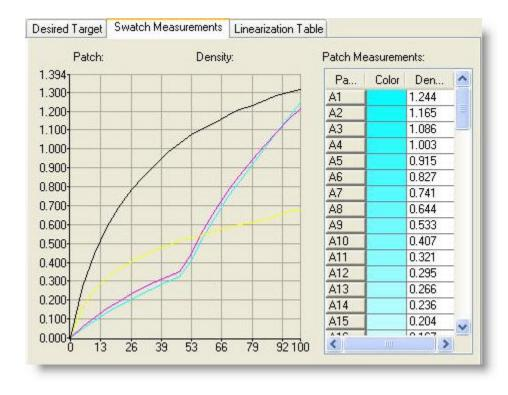
This issues displayed in the swatch measurement curves is indicative of the "Light" ink levels having a very light density scale in relationship to the "Dark" ink level.
