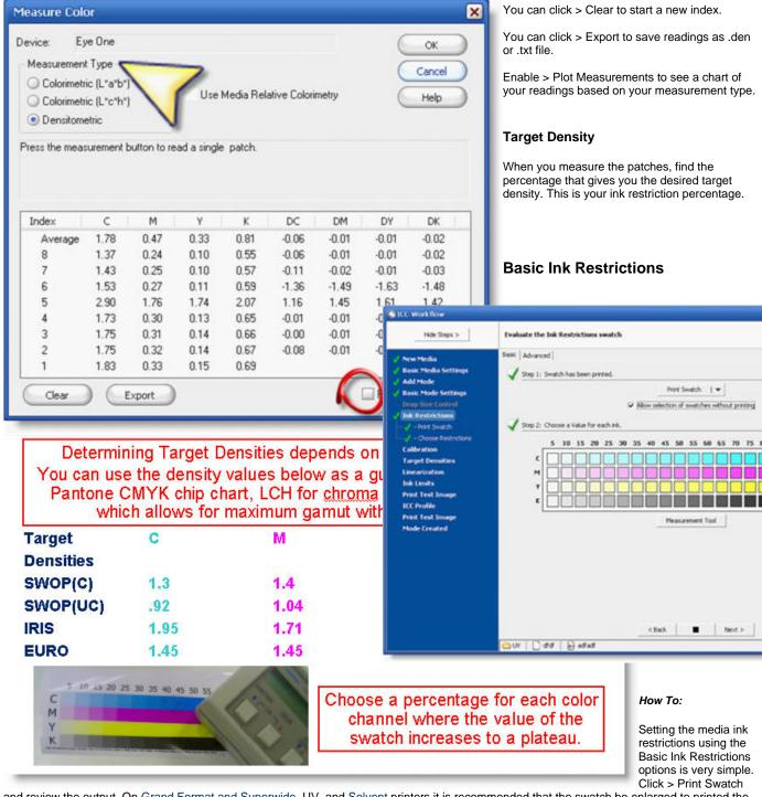
and review the output. On Grand Format and Superwide, UV, and Solvent printers it is recommended that the swatch be enlarged to printed the full width of the printer, or that enough copies are printed to allow the printer to come up to full production speed and temperature, etc.
