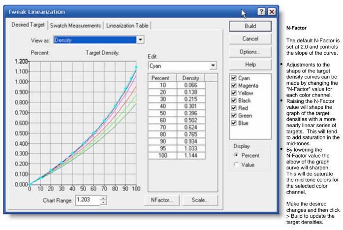
Print a test image and compare to a known proof to see if the adjustments are satisfactory. Don't worry about the overall total ink at this point because ink limiting can be adjusted in the next step. The primary reason we consider modifying the desired target curve is because some inks are non-linear, meaning that at 10% you may not be getting a true 10% work of ink.
