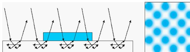
Figure 2 – Optical dot gain occurs when light entering ink is scattered by media causing dots to appear fuzzy and paper to appear darker.
